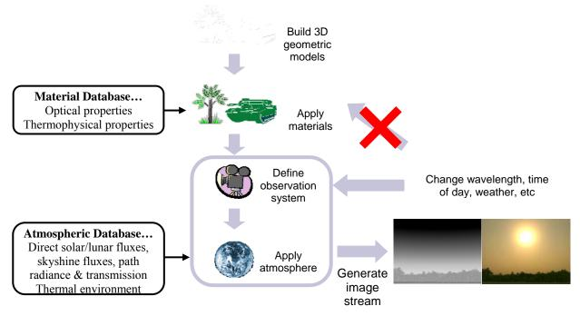
Figure 5. Flow diagram of the processes involved in producing CameoSim imagery
